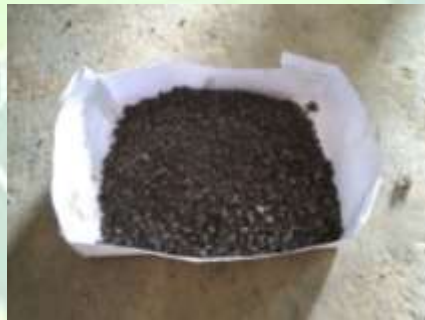
Gambar 3.11 Limbah Reclaimed Asphalt Pavement (RAP)
