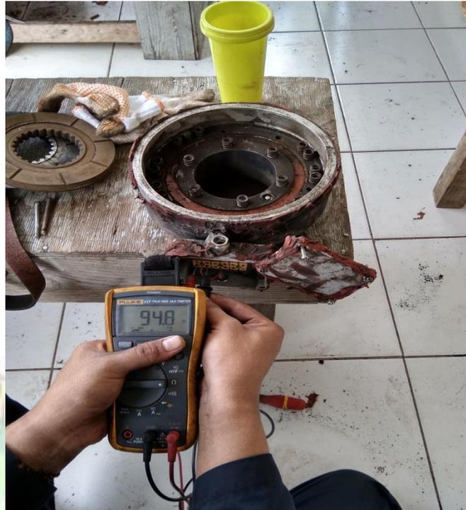
Gambar 4.3 Resistan Koil Brake Pad Motor 7
