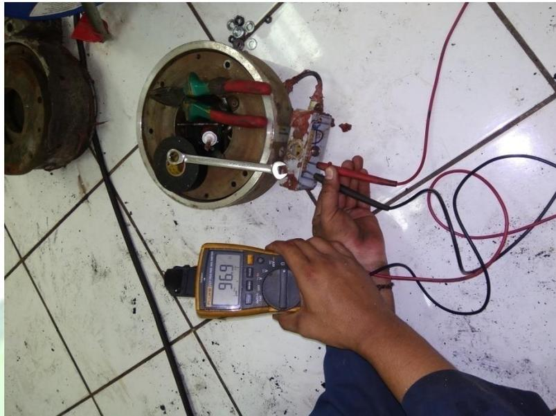
Gambar 4.2 Resistan Koil Brake Pad Motor 2
