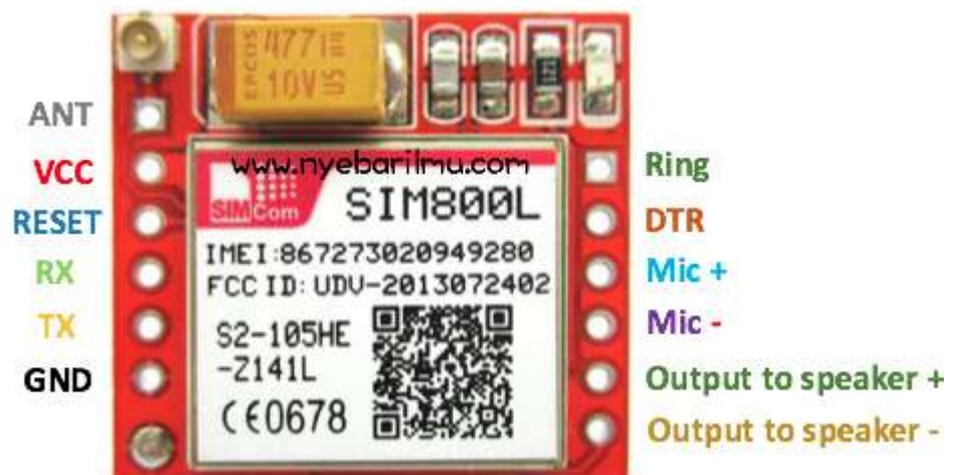
Gambar 2.25 Modul GSM SIM800L
