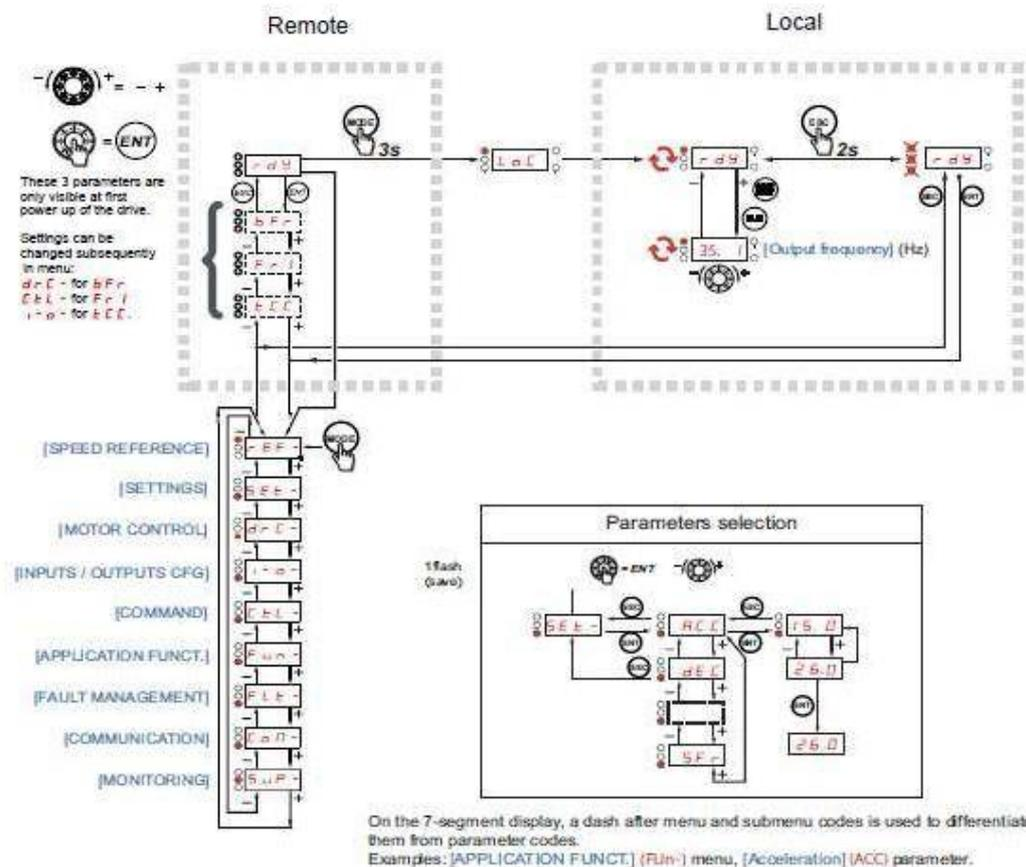
**Note:** The drive goes back to REMOTE configuration after a factory setting operation ([Restore config.] (FCS)) or by modifying the macro configuration ([Macro configuration] (CFG)).
