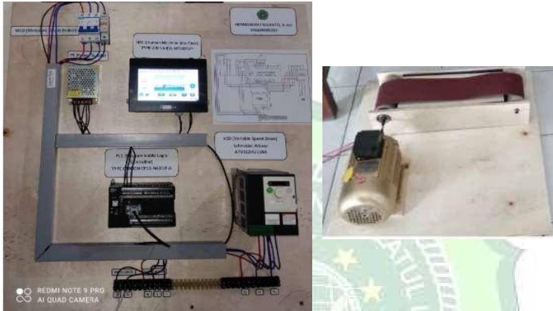
Gambar 4.14 Hasil prototype kontrol motor
